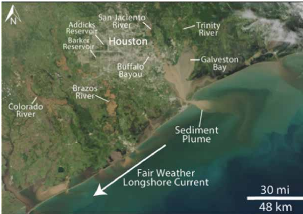
Figure 8. Satellite image of the Buffalo Bayou system and Texas Gulf Coast 4 days after Hurricane Harvey, at the end of the early adjustment phase (modified from Carlowicz and Allen, 2017). The brown water shows a sediment plume that overwhelmed the longshore current direction. The work of Ramon-Duenas and Wellner (2019) at the University of Houston focuses on understanding the sediment transport and the coastal responses to storms in the flood tidal delta. Their pre- and post-Harvey data at San Luis Pass provides hints at how the area responds to storm episodes. San Luis Pass is just northwest of the trailing end of the arrow labeled “Fair Weather Longshore Current.”
