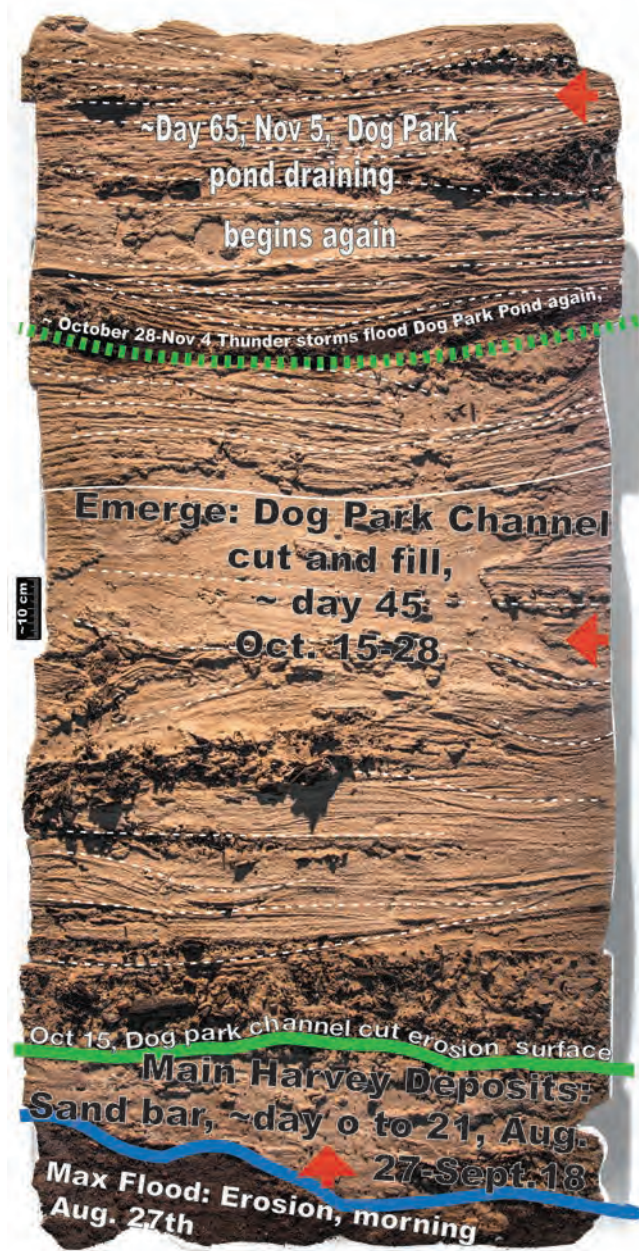
Figure 4a. Interpreted sand peel sculpture of the flood and adjustment phase Flood: The irregular sand on clay contact near the base of the sand peel records erosion at the peak of Harvey flooding early on the morning of August 27th (blue line). The approximately 6-inch-thick layer of finely structured sand records the waning flow of Buffalo Bayou during the next 20 or so days. This flood phase deposited thick a sand bar but only a thin remnant remains (blue to green line). The flow direction is away from the viewer. Adjustment: Approximately 45 days after Harvey, Buffalo Bayou dropped 10 feet (~3m), receding back to its channel, and water began to drain from a pond formed at the dog park. After ~ October 5th, the rapidly draining pond partially eroded the sand bar, then deposited the sand in the upper 4/5ths of the sculpture (above green line). This peel also captures an additional event from a thunderstorm in November that refilled the dog park pond and deposited a new layer of mud (dashed green line). This later drainage of the pond again deposited additional sand and debris in the upper 1/5th of the tapestry. For the adjustment period, (above green line) the flow direction is from right to left.
