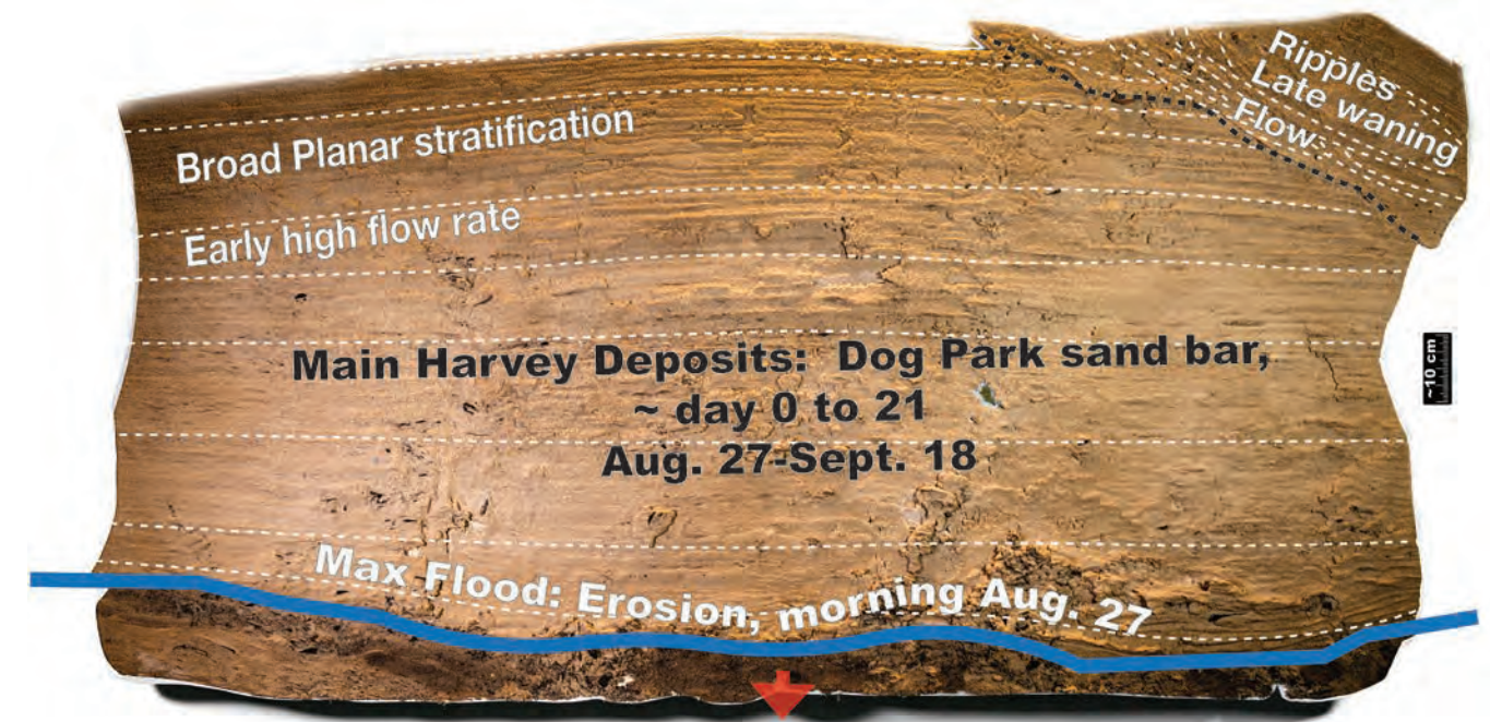
Figure 3a. Interpreted sand peel sculpture of the waning flood. Flood: The sand on clay contact near the base of the sand peel records erosion at the peak of Harvey flooding early on the morning of August 27th (blue line). The approximately 24-inch-thick broadly layered fine sand above the erosional base records the initial deposits from waning flow of Buffalo Bayou during the next ~20 days. In the upper right corner of the sculpture, above an erosional surface, are shorter wavelength bed forms and ripple marks interpreted to result from reduced flow rates. This phase deposited a sand bar up to ~12 feet (3.5m) thick. The flow direction of the bayou is towards the viewer. All the sand peel sculptures are shown as mirror images so the orientations are as they appeared in the outcrops. The red arrows indicate the net flow direction. Up arrow is for flow away from the viewer and a down arrow is toward the viewer.
